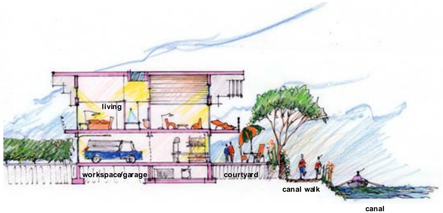
Live/Work Unit Section
